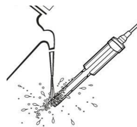
Figure 16: Rinse the probe with DI water
